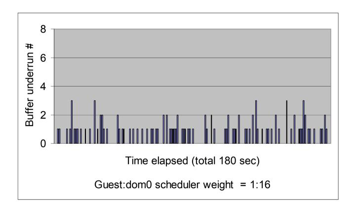
Scheduler tick, from 10ms default to 1ms, reduces average buffer underrun frequency from 2.47 per second to 0.594 for 1/17 CPU reservation
